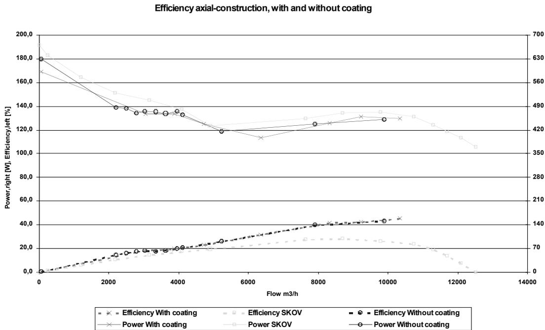
Figure 8: Efficiency, small ventilator
