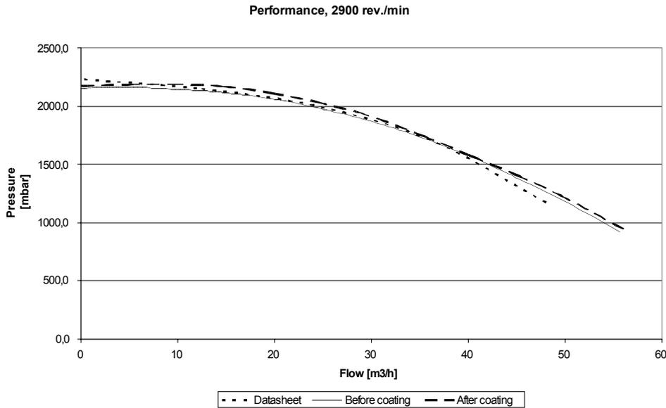
Figure 5. Pump performance, small low pressure new pump
