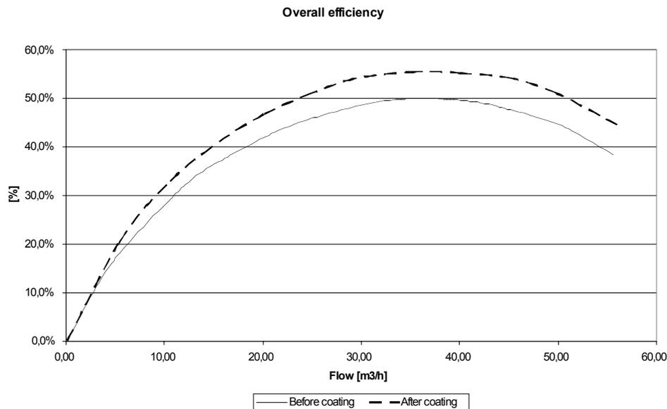
Figure 6: Overall efficiency, small low pressure new pump
