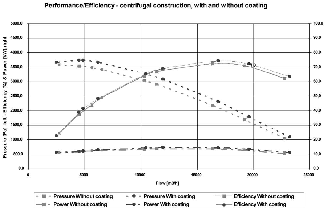
Figure 9: Performance & Efficiency, medium sized ventilator
