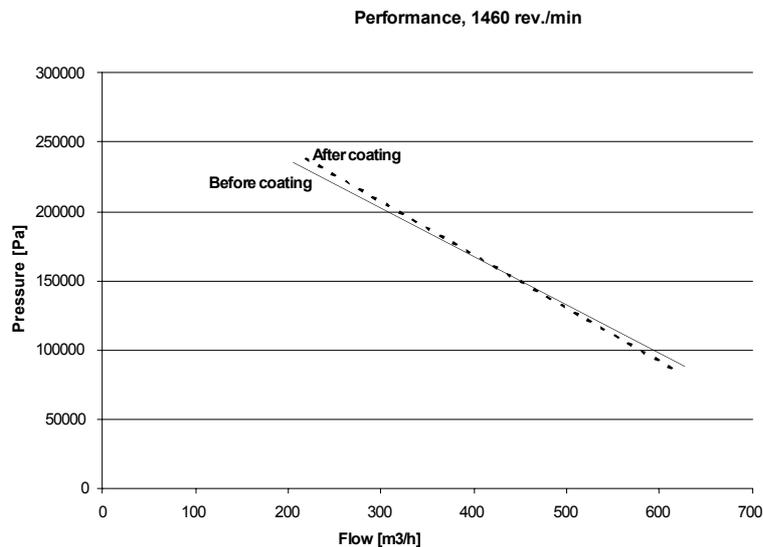
Figure 3. Pump performance, low pressure used pump / waste water
