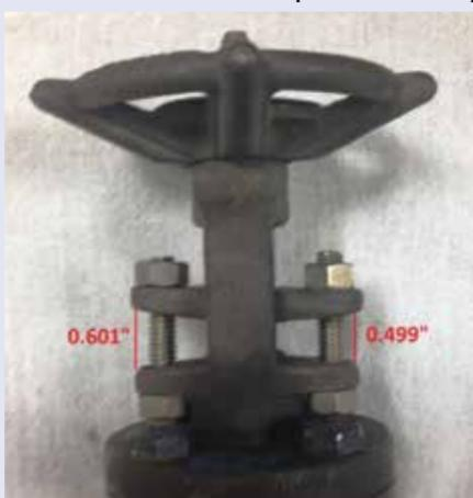
Figure 1. Uneven loading of gland flange
