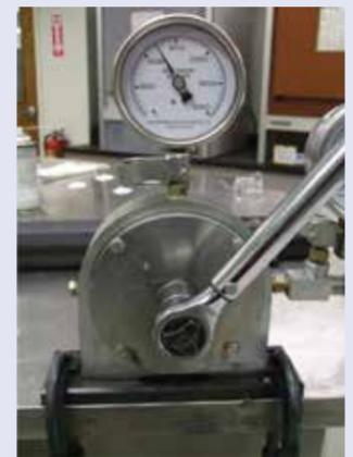
Figure 2. Thread lubricant tested for Knut factor friction variation
