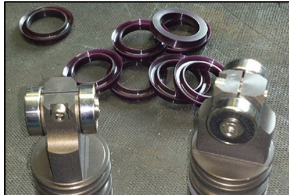
Pistons with P22KN Rod and Piston Seal with 19K Split Wear Rings.
