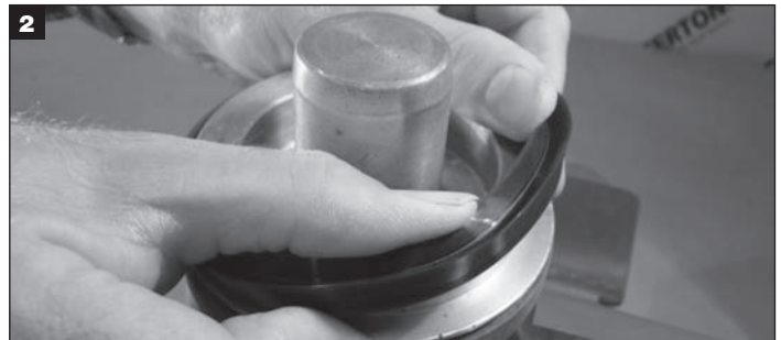
Hold piston securely, locate seal into groove and use finger pressure to begin stretching over piston head.
