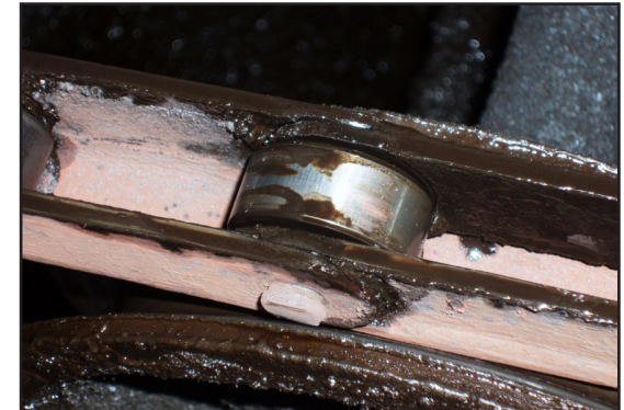
Chain rollers frozen from the old lubricant.
