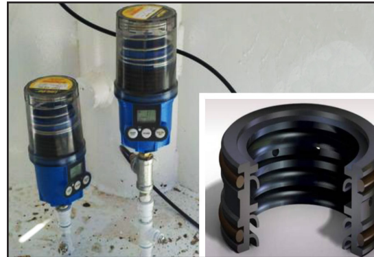
Chesterton Lubri-Cup™ EM and 615 HTG installed.
