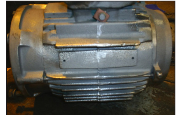
Cleaned electric motor after coating with ARC S4.
