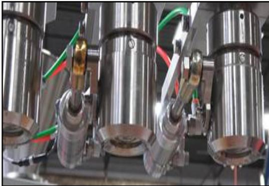
*Pneumatic actuators on filling machine.*
