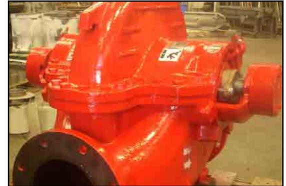
*Horizontal pump with 860 MPG applied.*
