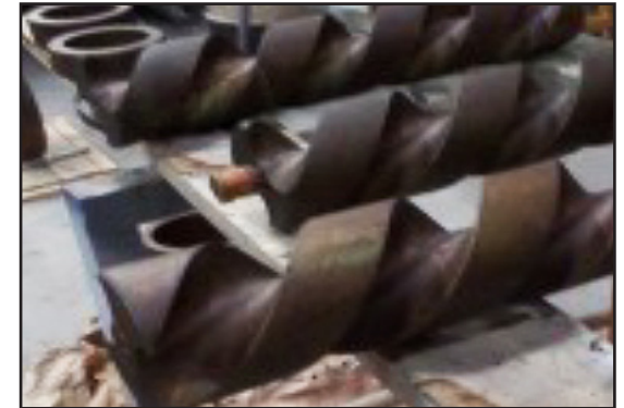
740 Heavy Duty Rust Guard leaves a dark brown, transparent waxy coating for up to 2 years' protection.
