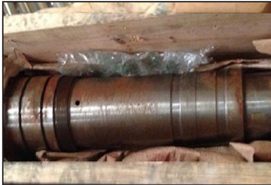
Rusted shaft taken from storage box using rust inhibiting paper wrap.
