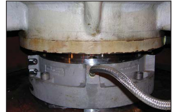
Chesterton large split seal installed.
