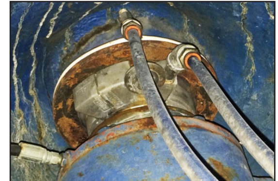
Stock chest agitator fitted with Chesterton 442C Split Seal.
