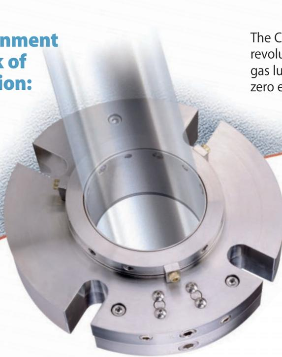
The CHESTERTON 4410 Hydrostatic Gas Seal is a revolution in gas seal technology. This coaxial, coplanar, gas lubricated dual seal offers the total containment and zero emission capability of conventional dual seals, but without risk of barrier fluid intrusion into the vessel. Operates from low to elevated speeds equally well, and with virtually no face wear and no resulting particulate contamination. The best new technology for hazardous, highly reactive or sanitary product.
