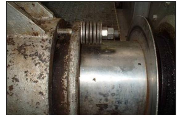
*Chesterton's 5150 Rotary Live Loading system avoids leakage by automatically maintaining the correct sealing force on the packing set.*
