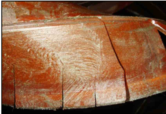
Lip of the failed seal
