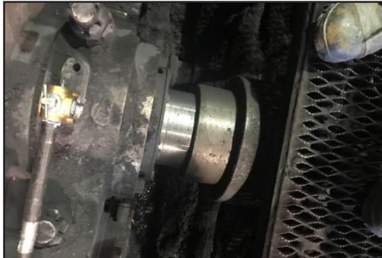
Rubber lip Seals were causing shaft wear.
