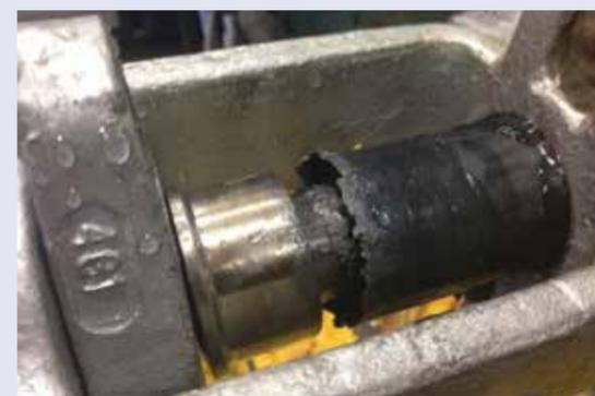
Figure 4. Low emission packing extrusion caused by excessive gland clearance.
