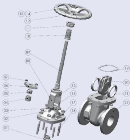
Figure 1. Typical components of an API 600 gate valve.
