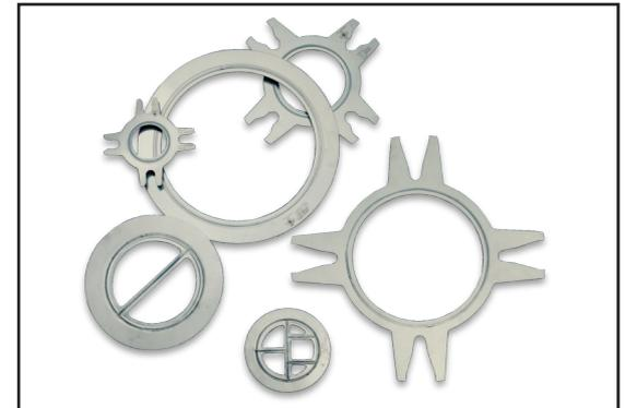
The Chesterton SteelTrap Gasket has concentric, isolated convolutions that trap pure graphite against the flange face
